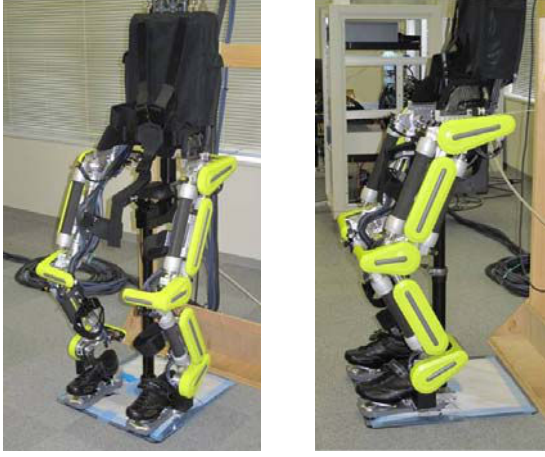
Fig. 1. Our newly developed eXoskeleton Robot (XoR)[12]. Height: 1.5 m, Weight: 30 kg. XoR has ten degrees of freedom and six active joints. Each active joint uses a hybrid actuator composed of air muscle and an electric motor. XoR is designed to assist lower-limb movements in humans.
