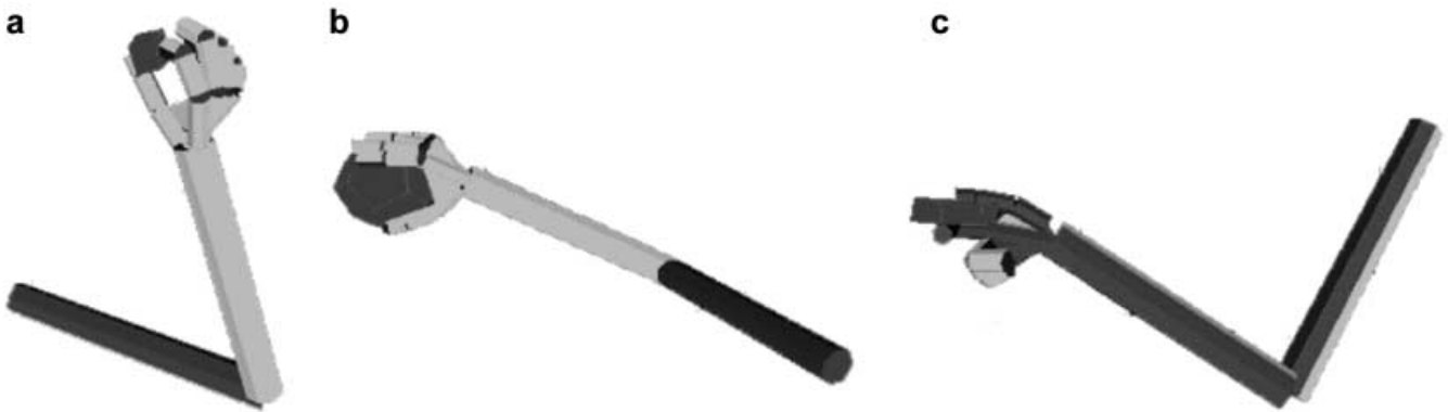
Fig. 8a–c. Grasps generated by the simulator: a a precision grasp; b a power grasp; c a side grasp
